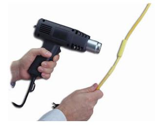
Position tubing over object and heat evenly until tubing shrinks into place or will shrink no further. Products containing pre-installed adhesive may need extra heat to melt and flow the adhesive for proper application.
